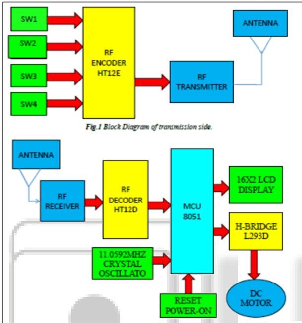
Fig.1 Block Diagram of transmission side.
