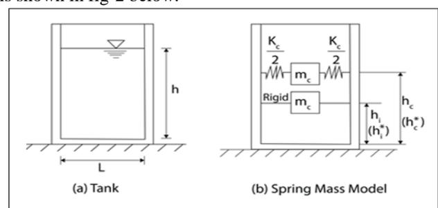
Fig. 1: Spring-Mass Model for Ground Supported Rectangular Tank
