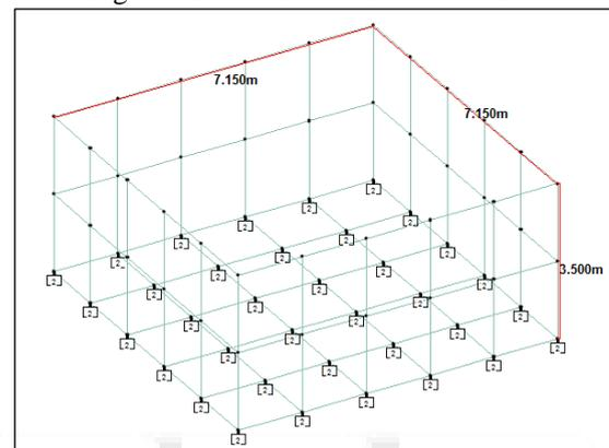
Fig. 4: Dimensional Model of Tank (Center to Center Dimension of Tank Wall)
