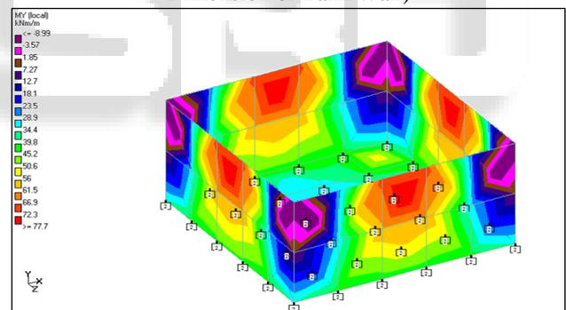
Fig. 5: Maximum Moments Results on Side Walls and Base Slab
