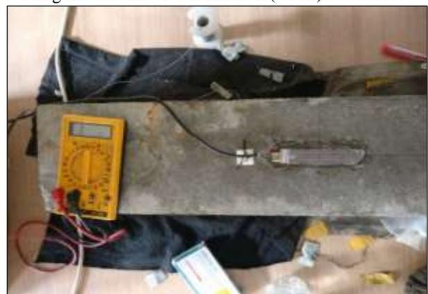
Fig. 6: Fixing of strain gauge
