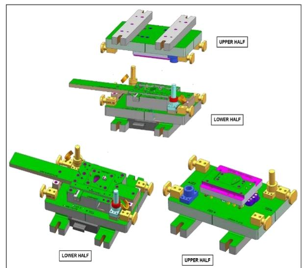
Fig. 5: Final Parts of Die Assembly
