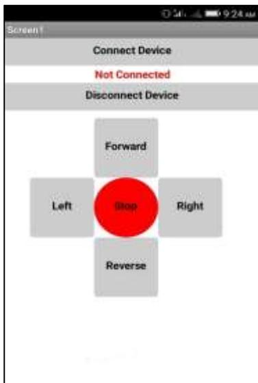
Fig. 2: shows the Manual Control Interface
