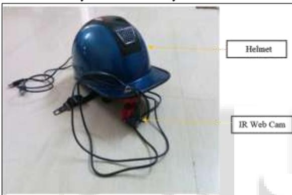
Fig. 1: IR Web Cam Attached with Helmet
