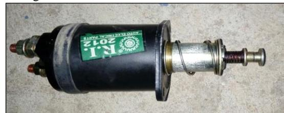
Fig. 3: Electromagnetic Actuator
