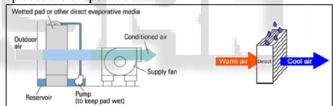
Fig. 2: Direct Cooling
