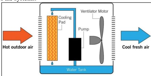
Fig. 1: Direct Evaporative Cooling System
