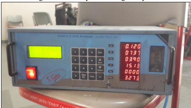
Fig. 8: Gas Analyser readings for mixture of petrol & hydrogen
