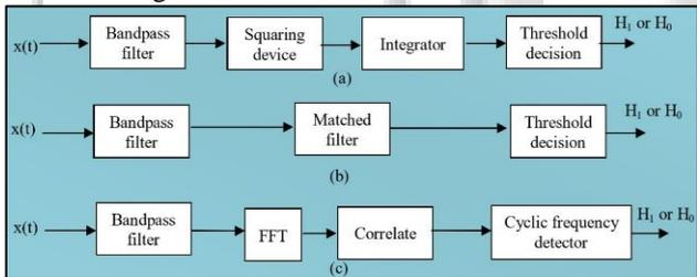
Fig 1: Block Diagrams For: A) Energy Detection; B) Matched filtering; C) Cyclostationary Feature Detection
