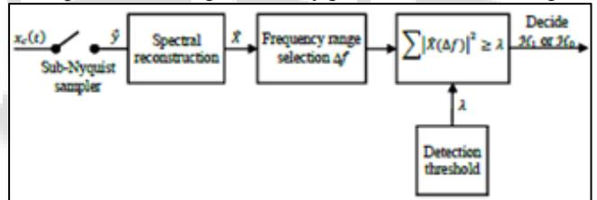
Fig 3: Block diagram for Sub-Nyquist wideband sensing
