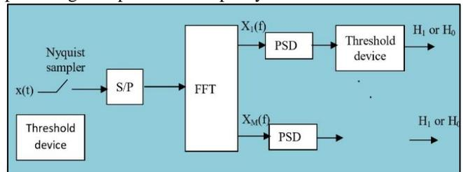
Fig 2: Block Diagram for Nyquist Wideband Sensing
