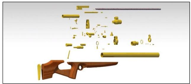
Fig. 6: Disassembled Rifle 3D printable parts
