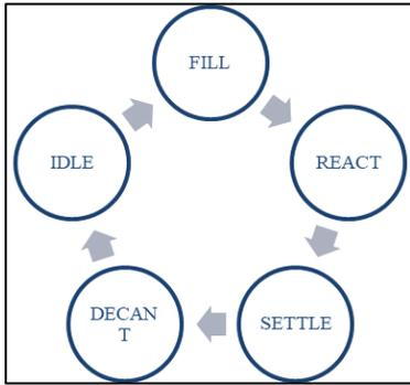
Fig. 1: SBR Operation for One Cycle
