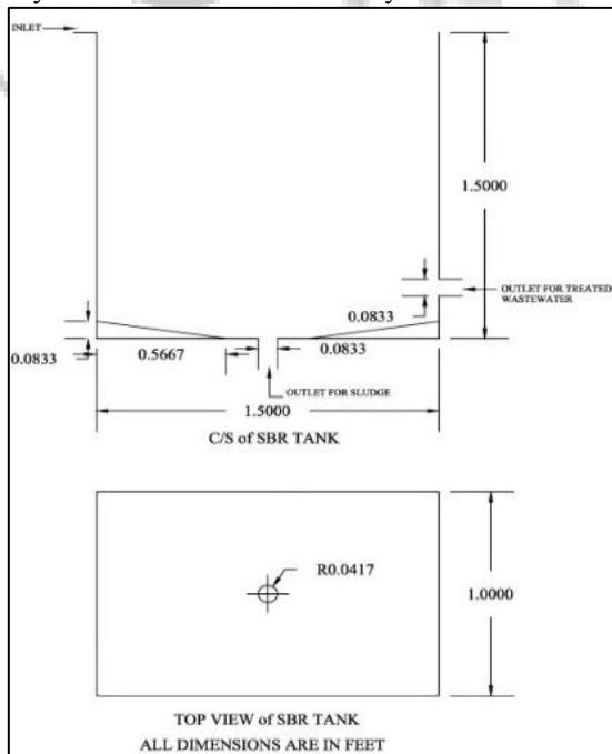
Fig. 2: Dimensions of Tank
