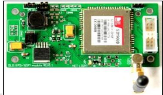
Fig. 4: GSM modem
