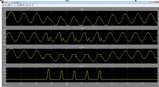
Fig. 5: Si Diode Based MOSFET Characteristic Simulation Result from Switching Circuit
