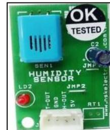
Fig. 3. HSM 20g Humidity Sensor
