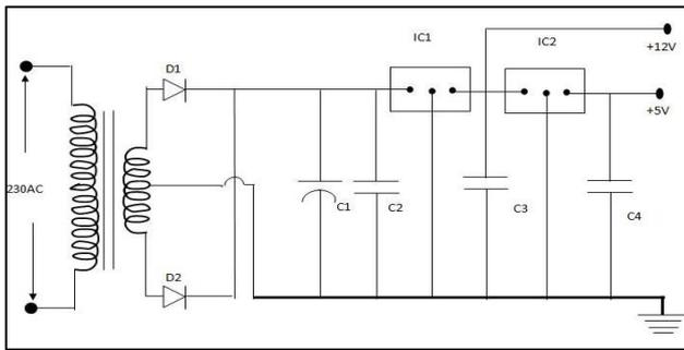
Fig. 7: Full Wave Regulated Power Supply
