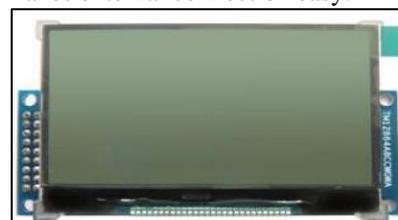
Fig. 6: GLCD 128X64 -TM12864A8CCWGWA
