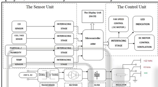
Fig. 1: Hardware Structure of the Indoor Air Quality Monitoring & Control System
