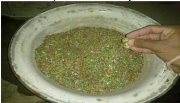
Fig. 1: Shredded Metalize Polymer Plastic
