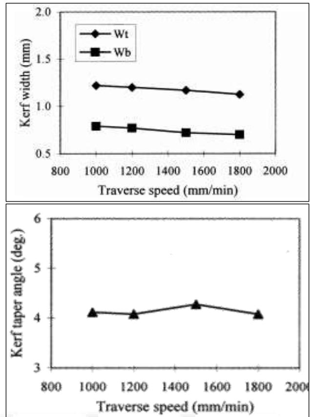
Fig. 8: The effect of traverse speed on the kerf geometry (water pressure=35 000 psi, stand-off distance=4 mm). Wang [12]
