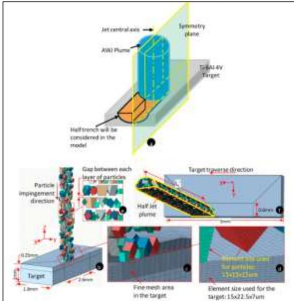
Fig. 3: (a) Symmetry of the AWJ milling process at 90° incidence angle. (b) 3D view of the model. (c) Meshing of the target and the particles. (d) Zoomed-in view of the elements used in the fine mesh area. (e) Gaps among the layers of the particles; in between these gaps the target will be traversed by some percentage of total distance to be covered across the jet. (f) Tilted top view of the model showing the length of the particles column.
