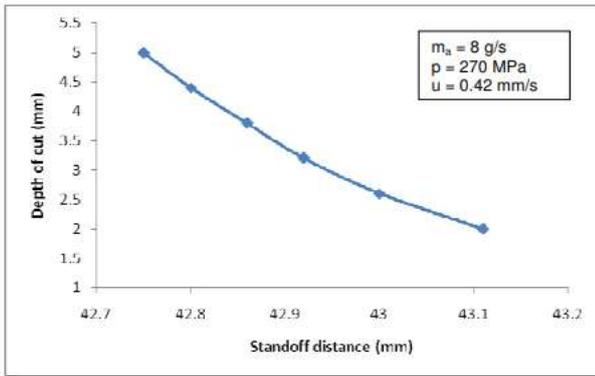
Fig. 2: Effect of standoff distance on depth of cut [5]
