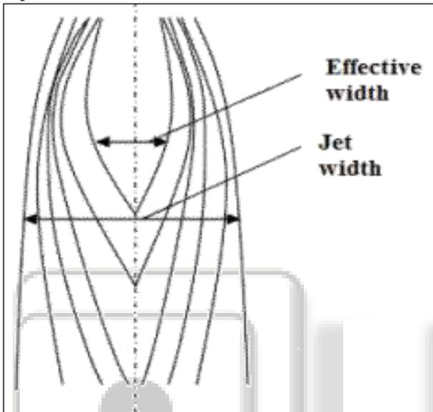
Fig. 6: Radial velocity distribution across the width of the nozzle [10]
