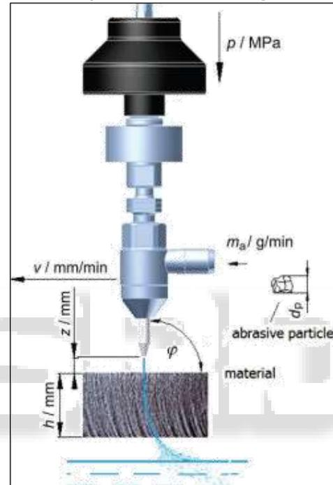
Fig. 1: Abrasive water jet cutting – water jet cutting head and process parameters
