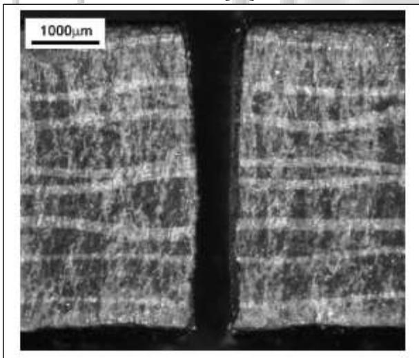
Fig. 7: Cross-section of Gr/Ep composites cut with abrasive waterjet: water pressure = 210 MPa, traverse speed = 30mm/s, standoff distance = 3mm, abrasive mass flow rate = 8.5 g/s. [11]
