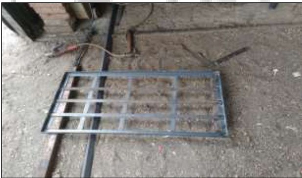
Fig. 4: Mild Steel Frame
