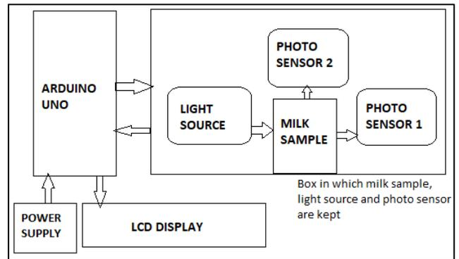
Fig. 1: Block Diagram of the Proposed Device
