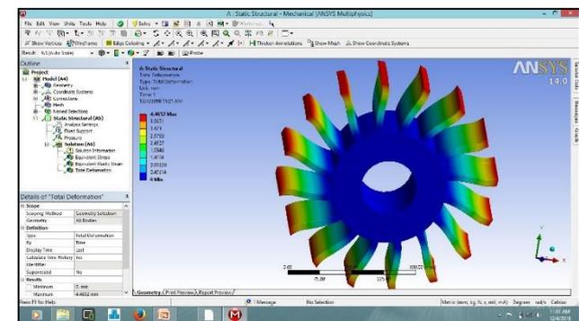
Fig. 9: (Static structural analysis of the impeller assembly for deformation)
