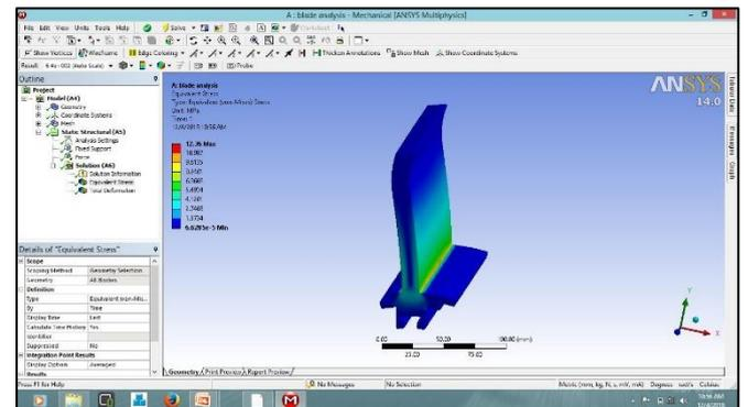
Figure 6 (Static Structural Analysis of the Blade For Stress)
