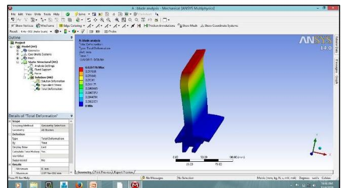
Fig. 7: (Static Structural Analysis of Blade for Total Deformation)
