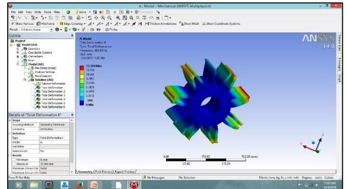
Fig. 10: (Model Analysis of the Impeller for Vibration)
