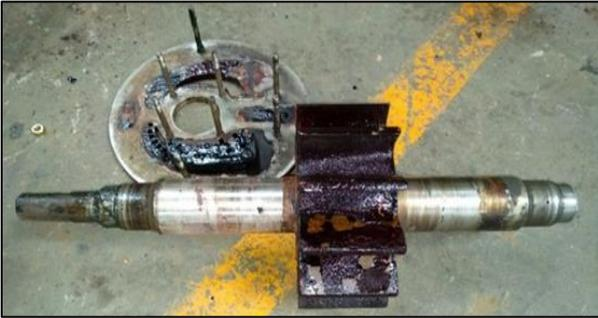
Fig. 1: (Damaged Impeller Blades by Chemical)
