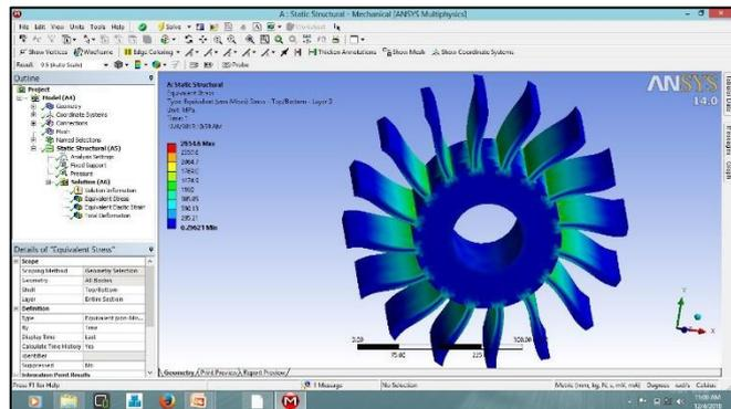
Fig. 8: (Static Structural Analysis of the Impeller Assembly for Stress)
