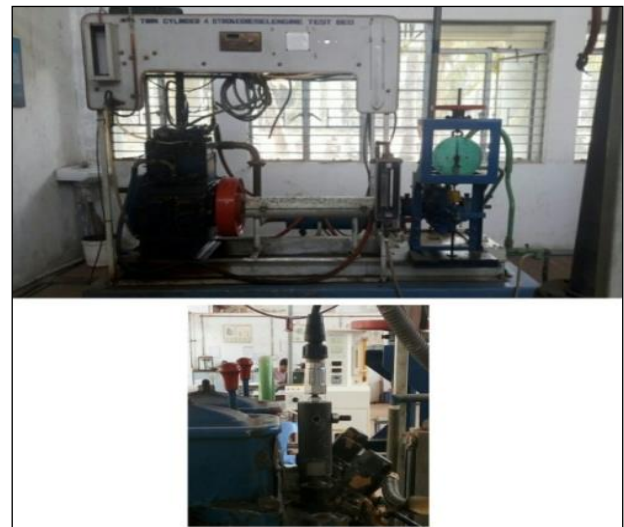
Fig. 1: Experimental test setup and position of accelerometer on cylinder head
