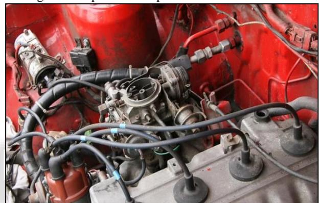
Fig. 2: Actual Setup of Modified Carburettor.
