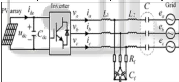
Fig. 2: three phase PV system with blocking capacitors
