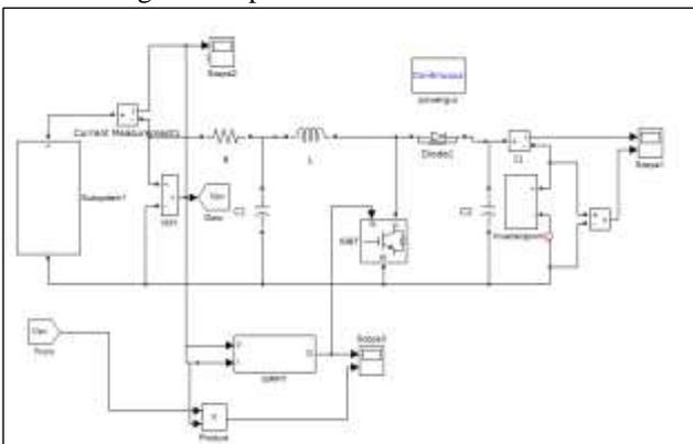
Fig. 7: MATLAB simulation of DC-DC boost converter with MPPT and Inverter
