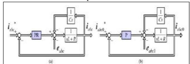
Fig. 4: (a) Current control loop in abc frame (b) direct current component control loop in abc frame
