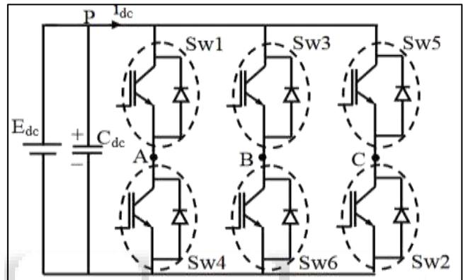
Fig. 2: Three phase voltage source inverter
