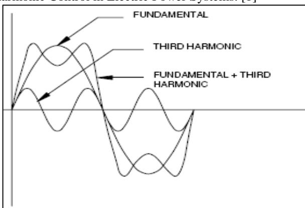
Fig. 1: Harmonic frequency waveforms
