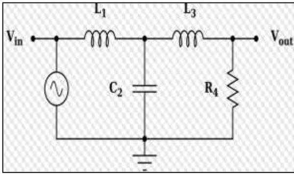
Fig. 3: LC Filter circuit
