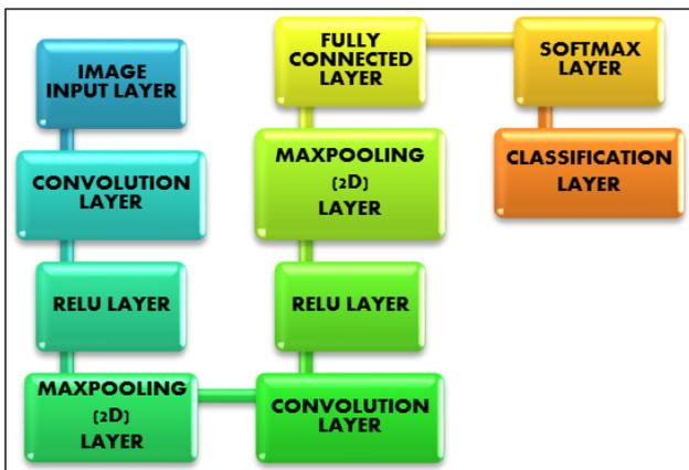
Fig. 3: Modified Convolutional Network Architecture
