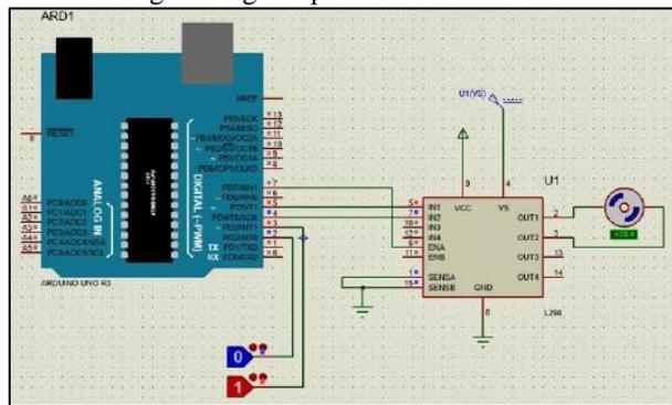
Fig. 4: Logic Input 2 Is Made “One”
