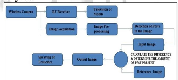
Fig. 2.4: Block Diagram of Pest Detection & Spraying of Pesticides
