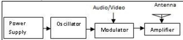
Fig. 2.2: Block Diagram of Transmitter
