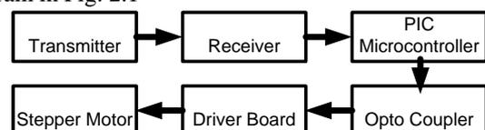
Fig. 2.1: Block Diagram of Robotic Motion
