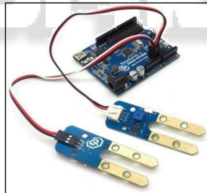
Fig. 4 Soil Moisture Sensors
