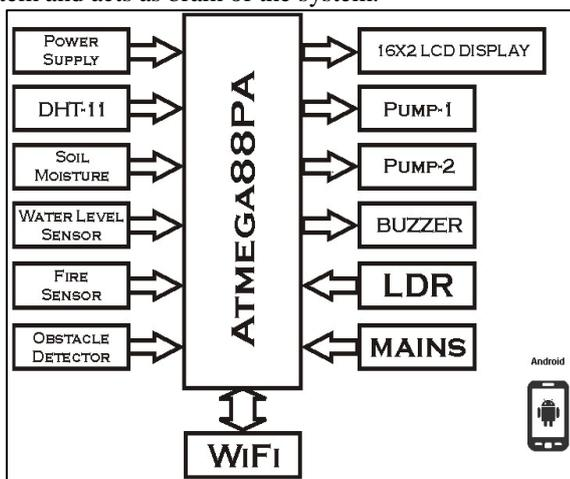
Fig. 1: Block Diagram of System Model
