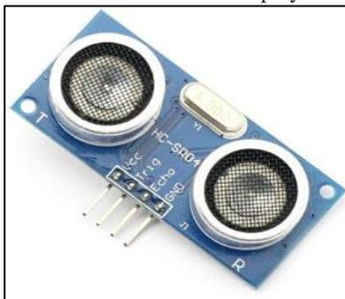
Fig. 6: Ultrasonic Sensor
