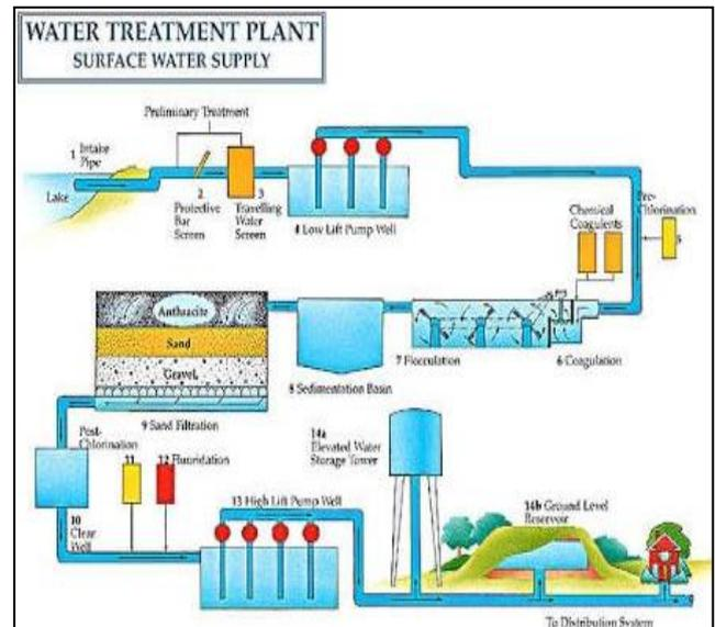
Fig. 1: The layout of Water Supply Scheme
