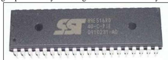
Fig. 4.1: SST Microcontroller
