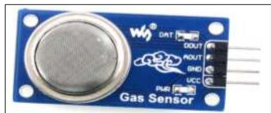
Fig. 4.2: MQ-2 Smoke sensor
