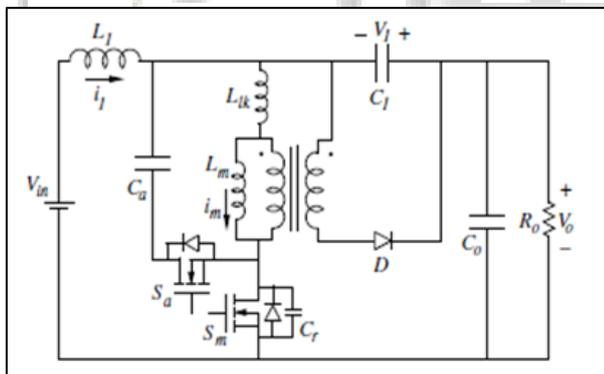
Fig. 3: Converter Circuit Diagram
