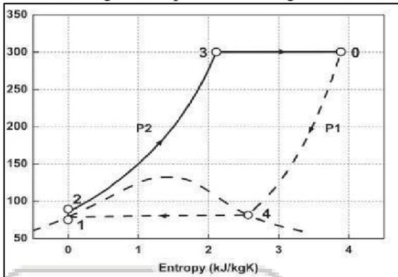
Fig. 5: T-S diagram of Engines Liquid Air Engine
