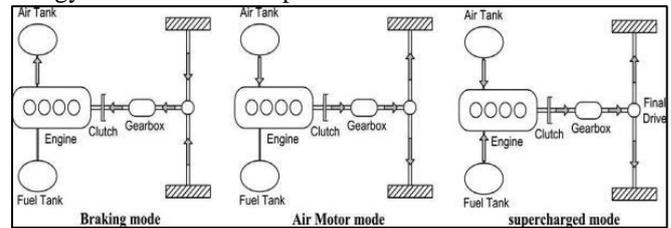
Fig. 4: Energy Flow at Different Operational Mode
