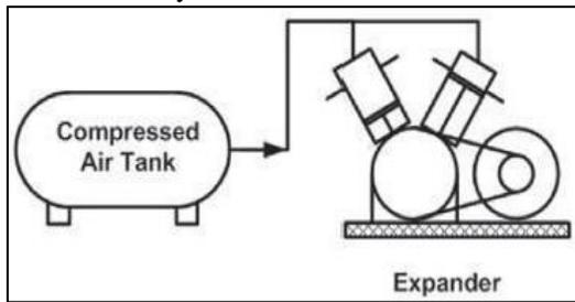
Fig 4: Compressed Air Engine
