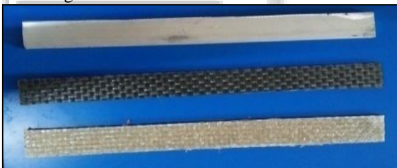
Fig. 2: Tensile Test Specimen
