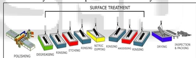
Fig. 1: Anodizing process
