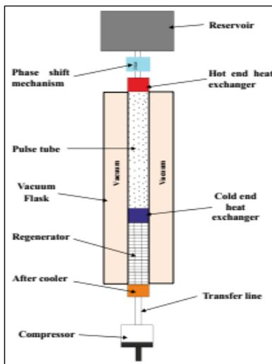
Fig. 1: Schematic of Inline Pulse Tube Cryocooler
