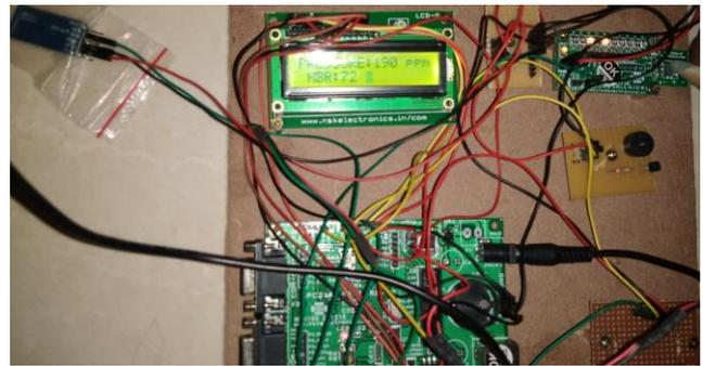
Fig. 3: Hardware connection setup for ICU patient monitoring system using Bluetooth module
