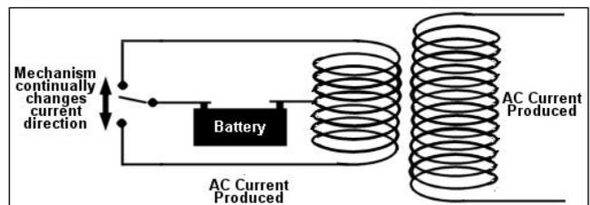
The output of this type of a circuit is a square wave.
