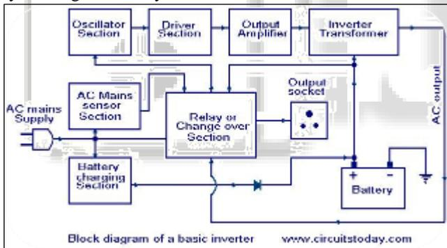
An inverter refers to a power electronic device that converts power in DC form to AC form at the required frequency and voltage output.
