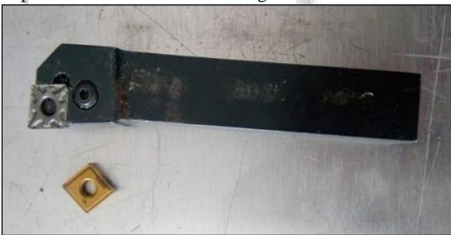
Fig. 1: Tool- Cemented Carbide Coated Insert
