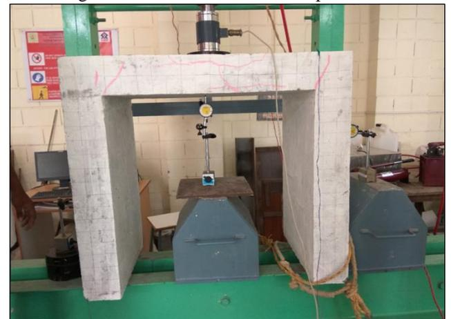
Fig. 9: Flexural failure at bottom of slab and shear failure at support
