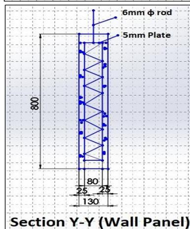
Fig. 1: Rigid Frame with 'W' connection (Wall Panel)
