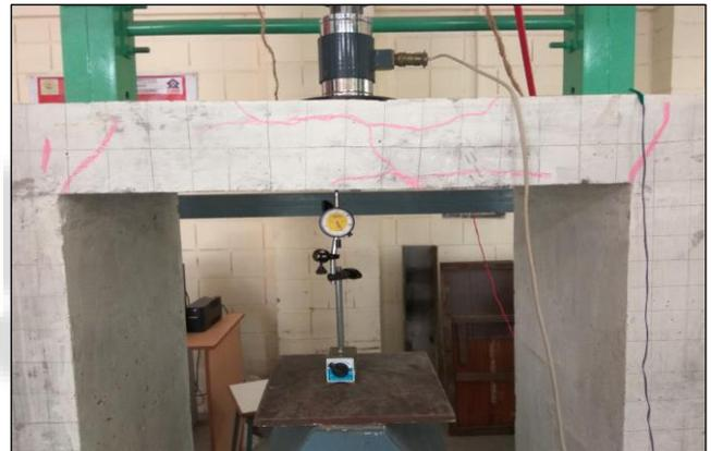
Fig. 8: Flexural failure at the roof panel slab
