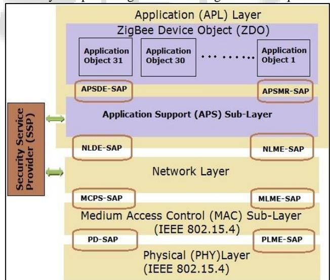
Fig. 4: Layer Architecture of ZigBee
