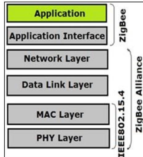
Fig. 3: ZigBee Protocol Stack
