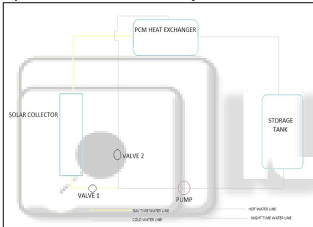
Fig. 3.1: Outline of thermal energy storage with solar water heater
