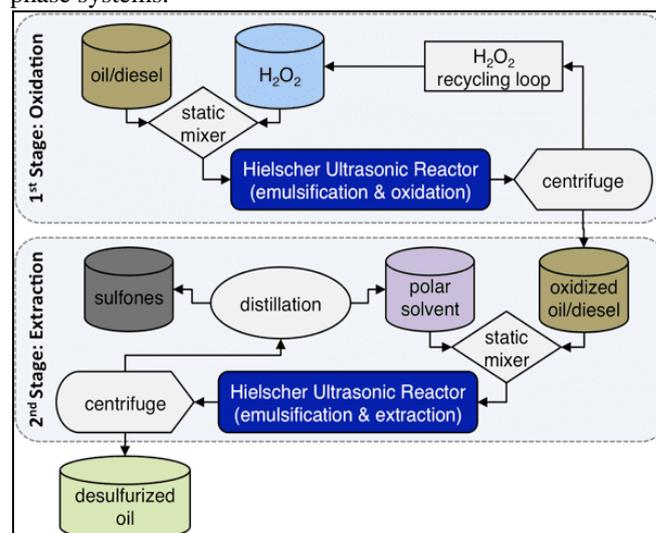
Fig. 2: Flowchart for Ultrasonically Assisted Oxidative Desulfurization – 2 Stages
