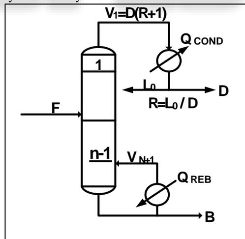
Fig. 3: A conventional distillation column.
