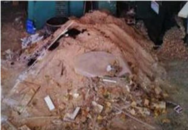
Fig. 2: Wastes generated during the processing of MDF and particleboard in furniture manufacturing.
