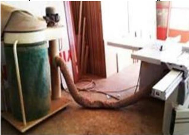
Fig. 3: Collection of dust generated during the cutting of wood by suction using a vacuum system
