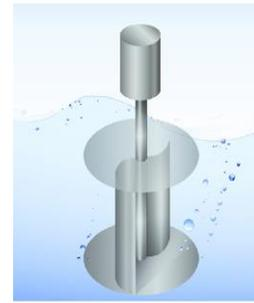
Fig. 6: Savonius turbine [8]
