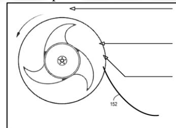
Fig. 7: rotor with deflector
