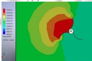
Fig. 11: External flow distribution pressure.
