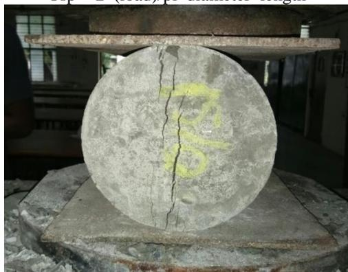
Fig. 10: 28-days Split Tensile Strength Test
