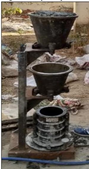
Fig. 5: Compaction Factor Test
