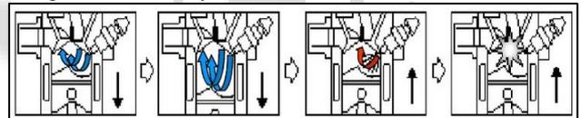
Fig. 1: Stratified Charge Engine
