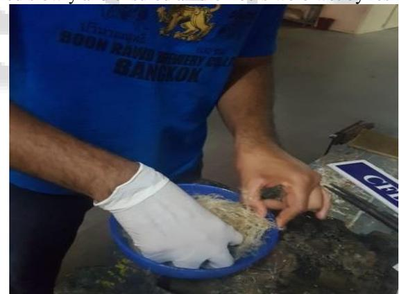
Fig. 5.3: Mixing Of Resin & Fibers
