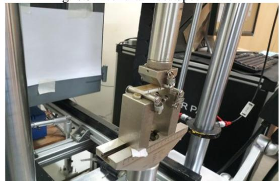
Fig. 6.4: Flexural Test
