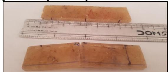
Fig. 6.3: Flexural Test Specimens
