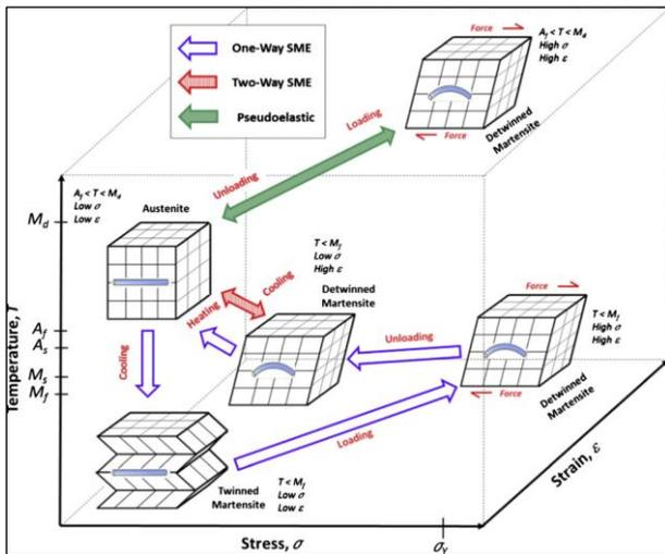
Fig. 1: SMA phases and crystal structures [3]
