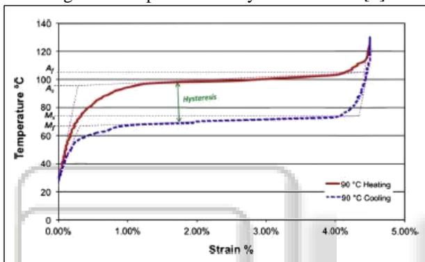
Fig. 2: Ni-Ti SMA phase transformation [3]
