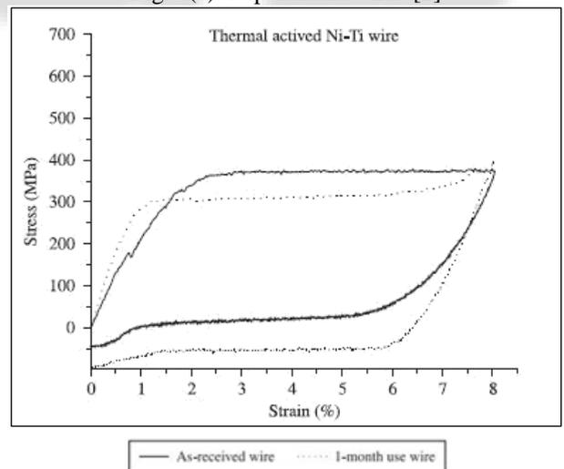
Fig. 3(b): Thermally activated wires [2]
