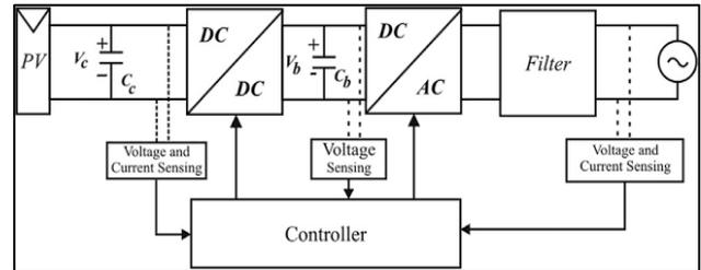
Fig. 1: Block Diagram of Standalone PV system
