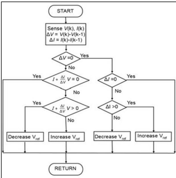
Fig. 3: Incremental Conductance Algorithm Flow Chart
