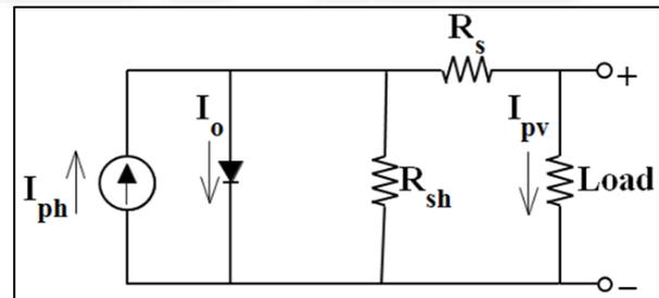
Fig. 2: Circuit Diagram of a Single PV Cell
