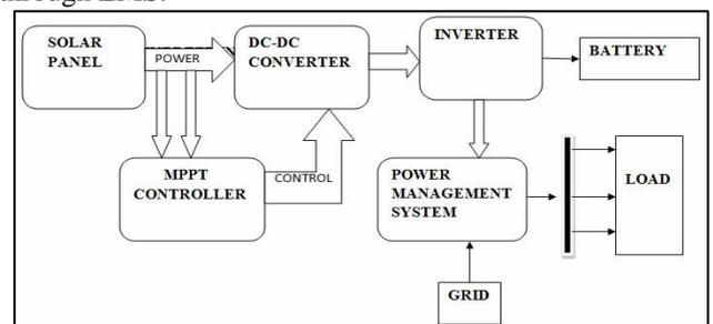
Fig. 6: Proposed Model Block Diagram
