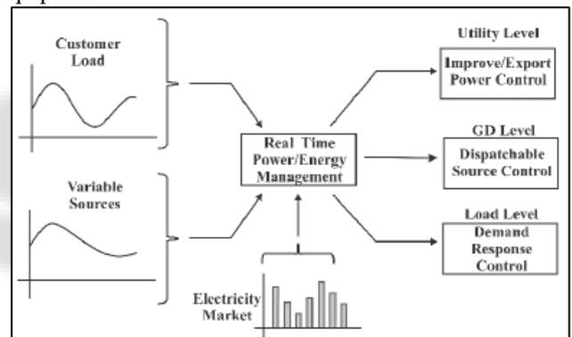
Fig. 5: Information Flow & Function of a real time EMS for microgrid
