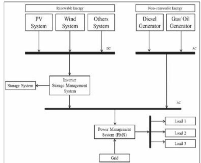
Fig. 4: Proposed Structure of Microgrid
